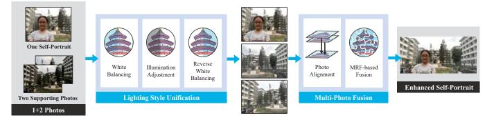
Fig. 1. Framework of the proposed multi-photo fusing method. Given one self-portrait and several supporting photos, our method first unifies their lighting style. A white balancing process is added to avoid color effects during the illumination adjustment and a reverse white balancing is performed to unify the color of the illumination. Then, the supporting photos are aligned to the self-portrait followed by a MRF-based fusion to nicely expand FOV of the self-portrait.
